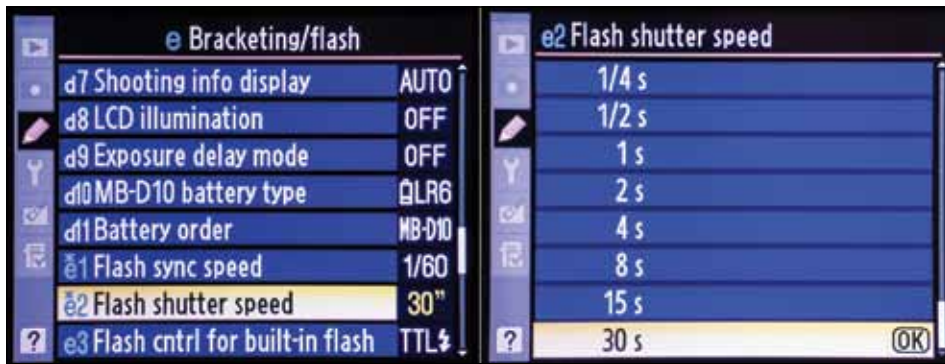
Figure 2. Camera menu #2: This shows two side-by-side views of the camera's menu for "Custom Settings" for selecting the slowest shutter speed that can be set when shooting with flash. Here, that shutter speed is set for 30 seconds.
