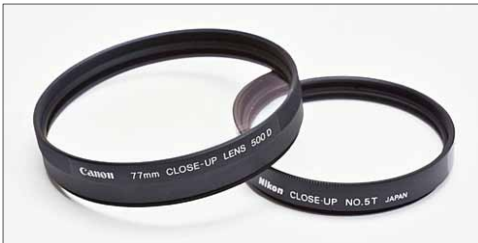
Figure 4. Close-up Lenses: These are close-up lenses manufactured by Canon and Nikon. The larger one is the Canon 500D and the smaller one is the Nikon 5T. The Canon close-up lens is available in 52, 58, 72 and 77 mm screw thread sizes and the Nikon is available in 62 mm. They attach to the front of a primary lens and allow that lens to focus much closer. Close-up lenses are also available from third party manufacturers for considerably less money, but they are also of lesser quality.
