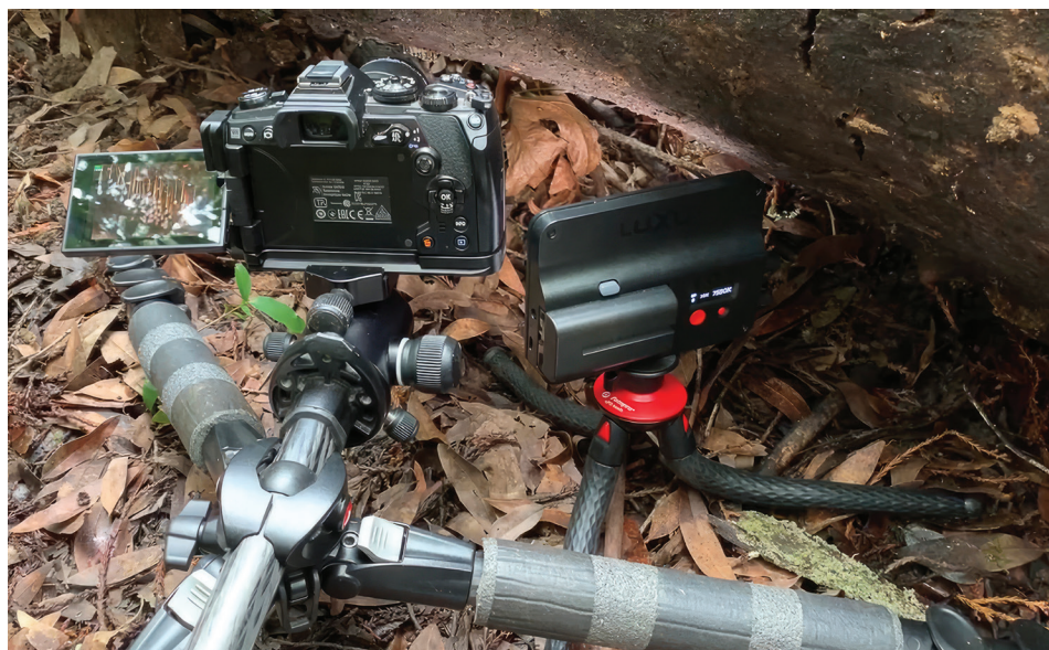
Figure 5. Getting the camera low to the ground with a tripod that has a center post that flips from vertical to horizontal.
