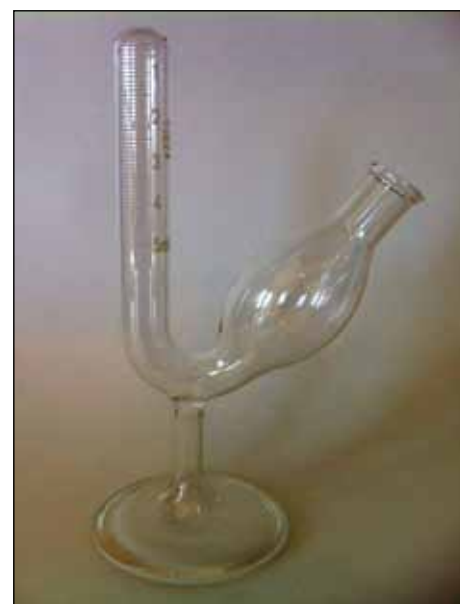
Figure 4. Graduated Durham Tube for fermentation studies.
