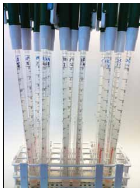
Figure 2. Volumeters used to measure volumes of CO 2 produced by yeast treatments.
